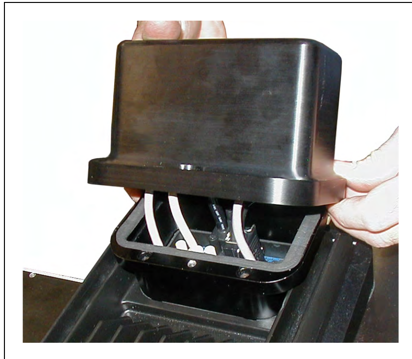
Figure 11-10. Installing Cable Entry Top Cover Assembly
